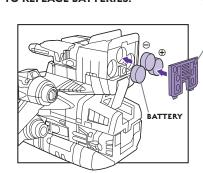
Using a Phillips/cross head screwdriver (not included), loosen screw in battery compartment door. Remove door. Remove and discard old batteries. Insert 3 x 1.5V "A76" or LR44 size alkaline batteries. Replace door and tighten screw. See diagram for polarity.
