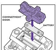
Using a Phillips/cross head screwdriver (not included), loosen screw in battery compartment door, Remove door, Remove and discard old batteries. Insert 2 x 1.5V "AAA" or R03 size batteries. Alkaline batteries recommended. Replace door and tighten screw. See diagram for polarity.
