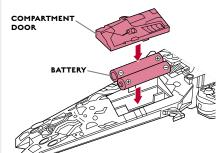
Using a Phillips/cross head screwdriver (not included), loosen screw in battery compartment door. Remove door. Insert 2 x I.5V "AAA" or R03 size batteries. Alkaline batteries recommended. Replace door and tighten screw.
