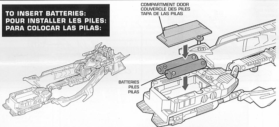
Using a Phillips/cross head screwdriver (not included), loosen screw in battery compartment door. Remove door. Insert 2 x 1.5 "AAA" or R03-size batteries. Replace door, and tighten screw with screwdriver. See diagrams for polarity.
