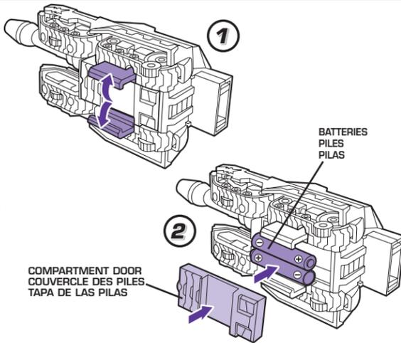
Using a Phillips/cross head screwdriver (not included), loosen screw in battery compartment door. Remove door. Insert 2 x 1.5 "AAA" or R03 size batteries. Replace door, and tighten screw with screwdriver. See diagrams for polarity.
