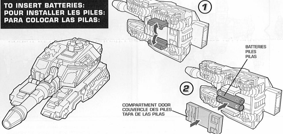
Using a Phillips/cross head screwdriver (not included), loosen screw in battery compartment door. Remove door. Insert 2 x 1.5 "AAA" or LR03 batteries. Replace door, and tighten screw with screwdriver. See diagrams for polarity.
